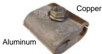
**#A41P - Bimetal Parallel Copper to Aluminum Splicer, Clamp Type**, made of cast aluminum and bronze inherently molded as one unit for splicing standard aluminum cable to copper cable through 2/0 size. Wt. .30 lb. ea.
