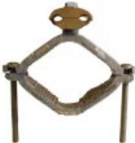
**#306B - Bronze Extra Large Perfection Pipe Clamp** with clamp type cable fastener that swivels 360 degrees. Fits from 2-1/2" to 4" iron water pipes. (Max. 4" O.D.). Tinned to prevent corrosion. Wt. 1.48 lb. ea.
