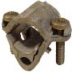
**#306 - Bronze Perfection Pipe Clamp.** Clamp type cable fastener, fits all standard cables through 2/0 and provides 1-1/2" contact with water pipes, rods, television masts, etc. Fits 1/2", 3/4" and 1" iron water pipes and 1/4", 1/2", 5/8", 3/4" and 1" copper water pipes. Wt. .48 lb. ea. \*
