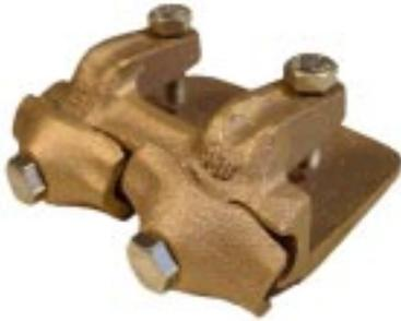
**#235X - Bronze Heavy Duty Beam Flange Bonding Connector** with 8 square inches of bonding surface. Ideal for bonding to flange of structural beams, columns and angles and steel purlins up to 3/4" thickness. Clamp type cable fastener fits all standard cables through 2/0. Requires no drilling, clamps direct to edge of steel. Wt. 1.60 lb. ea.
