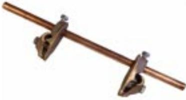
**#272W - Bronze Thru-Wall Connector** consists of 3/8" x 12" copper stem and two adjustable clamp type cable fasteners. Fits up to 10" thick wall. Longer stems can be furnished when specified. Wt. 1.16 lb. ea.
