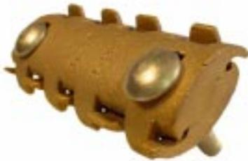
**#G27 - Bronze Large 4" All Purpose Connector** with two stainless steel 3/8" bolts, nuts and washers and used for connecting two cables or rods through 2/0 or 5/8" dia. Wt. .86 lb. ea. \*
