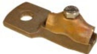
**#596 - Bronze Bus Terminal Metal Connector** with clamp type cable fastener for standard cables through 2/0. Fits over 1/2" bolt, for larger size bolt specify when ordering. Clamp has 5 sq. inches of bonding surface. Wt. .54 lb. ea. \*
