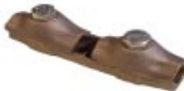
**#303 - Bronze Pressure Type Straight Cable Splicer** for connecting cables through 2/0. furnished complete with stainless steel hex bolts and washers. Bolt type cable action offers maximum strength. Wt. .58 lb. ea. \*
