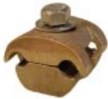
**#297A - Bronze Large Many Purpose Clamp** heavy duty, for clamping two standard cables through 2/0 and/or 1/2" and 5/8" rods. 2" long. Wt. .38 lb. ea.\*
