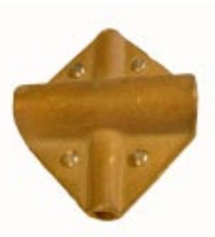
**#G95 - Bronze Large Heavy Duty Cross Run Connector** with hex-head screws. Measures 4" x 4" and used for bonding standard cables through 2/0 to 1/2", 5/8", or 3/4" dia. ground rods at right angles. When ordering, please specify size of ground rod and cable. Wt. 1.22 lb. ea.
