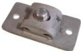
**#238B - Bronze Heavy Duty 2 Screw metal Bonding Plate** with clamp type cable fastener for all standard cables through 2/0. Affords 8 sq. inches of bonding surface. Wt. .66 lb. ea. \*
