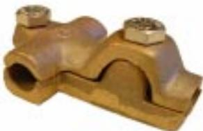
**#304 - Bronze Pressure Type "T" Cable Splicer** for clamping standard cables through 2/0. Furnished complete with two stainless steel hex bolts. Bolt type cable action offers maximum strength. Wt. .52 lb. ea. \*
