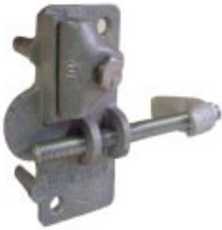
**#236 - Bronze Heavy Duty Metal Beam Connector** with 8 sq. inches of bonding surface, with clamp type cable fastener for standard cables through 2/0. No drilling required, fits 4" to 6" beams. If required for larger beams, specify size. Size may be varied by using different length bolt. Bolt clip casting must be formed over edge of beam. Wt. .98 lb. ea.
