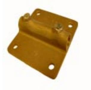
**#G88 - Bronze Extra Heavy Duty Large Bonding Plate**, 6" x 4-1/2" x 3/8" thick. For standard cables through 2/0. For use when an extra heavy duty large bonding plate is required. 27 sq. inches of bonding surface. Wt. 1.24 lb. ea.
