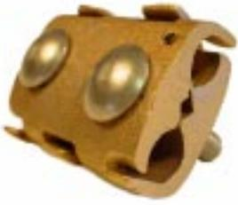
**#296 - Bronze Large Heavy Duty all Purpose Connector**, with two 3/8" stainless steel bolts, nuts and washers for connecting two cables or rods through 250m circular mills or 3/4" diameter. Wt. .80 lbs. ea.
