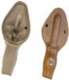
**#325 - Bronze Feed Thru-Roof Connector** with clamp type cable fastener furnished with two wood screws. Cable fastens underneath with finger type clamp and is fed down through roof or overhang. Underside is recessed and can be filled with plastic roof cement to afford perfect, weather tight seal. Wt. .72 lb. ea.
