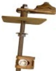
**#597X - Bronze Right Angle Thru-Roof Connector** consists of clamp type top cable connector, 4" square roof flashing plate, 1/2" x 8" threaded stem, hex nut and washer, and adjustable bottom clamp. Fits up to 6" roof thickness. If required for thicker roof, specify when ordering. Wt. 2.04 lb. ea.
