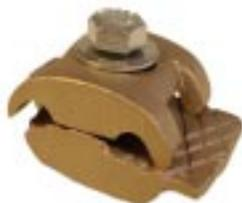
**#298A - Bronze Large Cable and Flat Iron Clamp** for connecting standard cable through 2/0 to angle iron, I Beams and flat iron strips. Also services as cable holder on I beams. Wt. .40 lb. ea. \*
