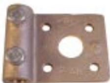
**#238 - Bronze Heavy Duty Bonding Plate** with 8 sq. inches of bonding surface. Fits up to 3/4" diameter bolt, for standard cables through 2/0. Wt. .78 lb. ea.
