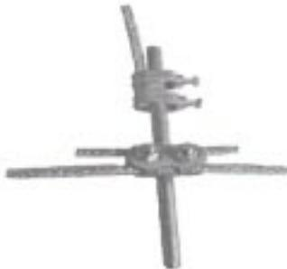
Detail view displays #51 Ground rod clamp on ground rod with cable and #28U U bolt Clamp, connected to a simulated counterpoise ground system. #28U is not intended to be the primary connections but is used as a secondary clamp for connection between a ground rod and counterpoise. Use of a ground clamp is necessary to meet UL requirements.
