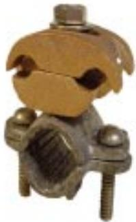
**#306CX - Small Copper Pipe Clamp** with bolt-type cable fastener that swivels 360 degrees. Fits maximum size 3/4" copper pipe. By inverting lower casting, clamp fits 1/4", 1/2" and 5/8" copper pipes. Tinned to prevent corrosion. Wt. .62 lb. ea.
