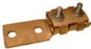
**#347 - Bronze Heavy Duty Bus Terminal** with 6" of surface contact for connecting two cables up to 4/0 size or 5/8" dia. to metal surfaces. Hole diameter are for 1/2" bolts. Cable fastener is two bolt style. Wt. 1.12 lb. ea.
