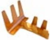
**#34L - Standard "T" Splicer** made of pressed copper. Gripping strength 260 pounds. 2" wide x 2-1/2" long. Wt. .12 lb. ea. \*
