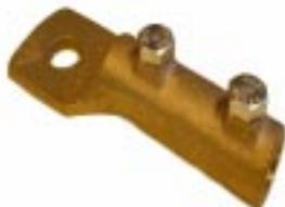
**#596A - Bronze Extra Heavy Bus Terminal.** 3 sq. inches of surface contact, for connecting 4/0 size cable to columns or larger metal bodies. Specify cable size when ordering. Standard hole size for 1/2" bolt but furnished for larger bolt when specified. Wt. .68 lb. ea.
