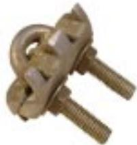
**#28U - Bronze 2" All Purpose U Bolt Clamp.** This part is used in conjunction with ground rod clamps for connecting to counterpoise ground systems. May be used for one or two horizontal cables through 2/0 and to rod up to 3/4" diameter. Clamp adjusts to various size cables and includes stainless steel nuts and washers. Wt. .62 lb. ea. \*
