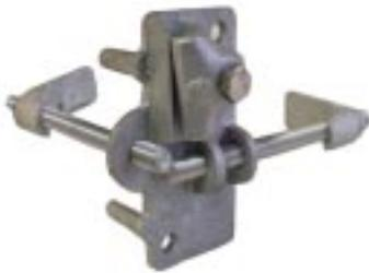
**#237 - Bronze Heavy Duty Angle Iron Connector** with 8 square inches of bonding surface, with clamp type cable fastener for standard cables through 2/0. Bronze bolt clip must be formed over edge of beam. Fits 2" to 4" size angles. (Reverse bolt clip for 2" size). Connector fastens directly to metal, no drilling required. For larger beams, specify size when ordering. Wt. 1.37 lb. ea.
