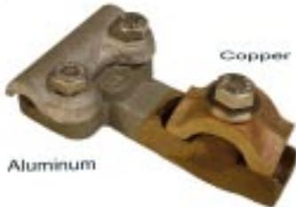
**#A304A - Bimetal Aluminum to Copper "T" Splicer**, Clamp type, made of cast aluminum and bronze inherently molded as one unit for splicing standard aluminum cable to copper cable through 2/0 size. Wt. .58 lb. ea.
