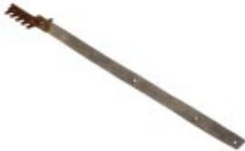
**#118 - Vent Pipe Bonding Strap**, for 2", 3" and 4" soil pipe. Cable connection for standard cables. Made of soft copper, tinned. Wt. .42 lb. ea.
