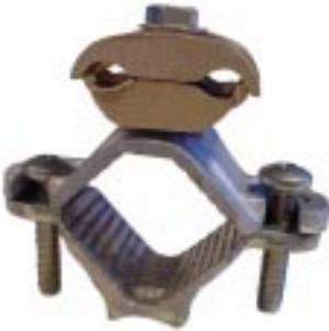
**#306A - Bronze Large Perfection Pipe Clamp** with clamp type cable fastener that swivels 360 degrees. Fits 1-1/2" and 2" iron water pipes. (Max. 2-1/2" O.D.). Lower casting may be inverted to fit smaller diameter pipes and rods. Tinned to prevent corrosion. Wt. 1.04 lb. ea.
