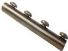
**#290 - Small Bimetal Straight Splicer** made of stainless steel for splicing miniature aluminum and copper cable. Fits No. 4 or No. 6 size cable. Wt. .14 lb. ea.
