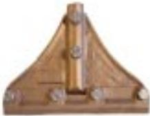
**#G181 - Bronze Heavy Duty Three Way Connector** for 1/0 or 2/0 cables with bolt type cable connection used for "T" cable splice on roof and for connecting to counterpoise cable. Eliminates right angle connections. Connector has 8" of contact with horizontal cable and 4" of contact with vertical or branch conductor. Wt. 2.10 lb. ea.
