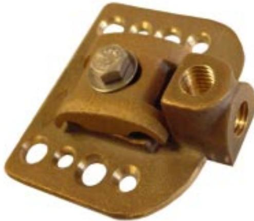
**#60U - Universal Mounting Base.** This base can be used for vertical or horizontal mounting. Base is threaded for 3/8" inside threads. Made of bronze material for pasterdown or fastening with screws for hammer drives. Wt. .80 lb. ea.
