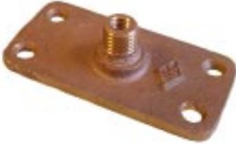
**#179 - Bronze Flat Metal Point Connector** with 8 sq. inches of bonding surface. Has 3/8" inside and 5/8" outside threads. Wt. .42 lb. ea.
