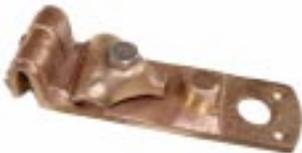
**#230 Bronze Gravel Stop Point Base** with 3/8" inside and 5/8" outside threads for fastening to gravel stop at roof edge. Wt. .02 lb. ea.
