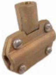
**#261 - Bronze Heavy Duty "T": Connector** with 1/2" inside thread and 4-screw clamp type cable connector. 5/8" inside thread available upon request. Wt. .82 lb. ea.
