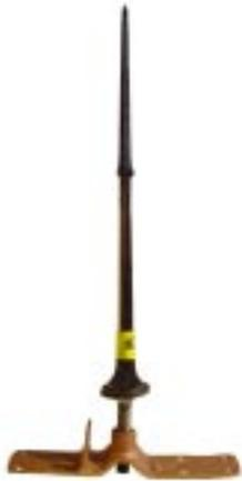
**#276 - Bronze Concealed Saddle Top** with 10" nickle plated air terminal (240A), 3" long threaded stem, stainless steel nut and washer, neoprene washer and saddle. Wt. .48 lb. ea.
