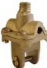
**#60SS - Bronze Base for Standing Seam Metal Roof.** Cable can be run parallel or perpendicular to seam. No penetration of roofing seam required. 5/8" outside and 3/8" inside threads. Wt. .93 lb. ea.
