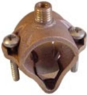
**#181 - Bronze Railing Bracket** with 5/8" outside and 3/8" inside threads with clamp style cable fastener. Fits up to 1-3/4" O.D. railing. Available with 3/8" inside thread upon request. Wt. .74 lb. ea. \*
