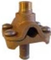
**#60A - Bronze Flat Surface Point Base** with 5/8" outside and 3/8" inside threads with 5/16" lead anchor and screw. The base requires only one anchor for fastening. Wt. .68 lb. ea.
