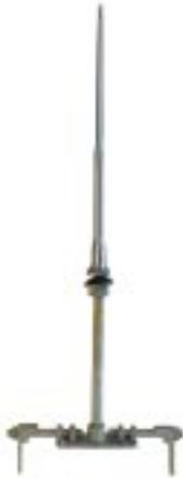
**#244 - Bronze Heavy Duty Metal Beam Air Terminal** with 8 sq. inches of surface contact, 10" nickel tipped point and neoprene washer. Standard clamp fits 4" to 8" beam. Reverse bolt clip for 4" size. Standard length of stem 8". (If clamp is required for larger size beam or if a longer stem is required, please specify when ordering.) Wt. 1.84 lb. ea.
