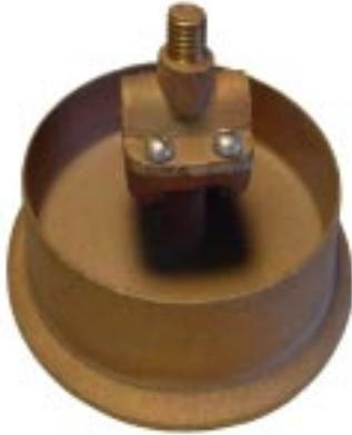
**#266B - No Nail Bronze Pan-Type Air Terminal and Cable Fastener Base.** Threads are 5/8" O.D. Base is fastened to roof with adhesive and then filled with stone, chips or concrete. Overall dia. is 4" and inside dia. of the pan is approximately 3-1/2". Wt. 2.90 lb. ea.
